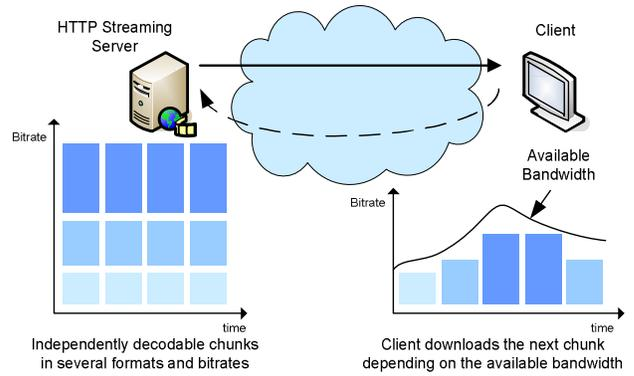
Fig. 1. Adaptive Bitrate Streaming Principle
