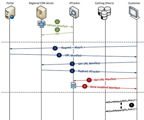
Fig. 3. Adaptive Streaming in a dCDN/CDN world
