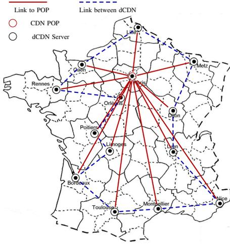
Fig. 5. Simulated dCDN topology; the cost of using an external (red line) link is twice the cost of using a peering (blue dashed line) link.
