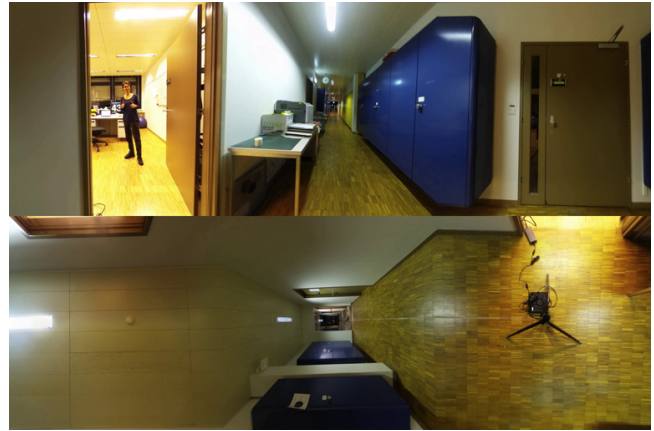
Figure 2: Example of omnidirectional video frame in cube-map baseball layout : the spherical frame is mapped to the plane via the cube-map projection and the faces of the cube are arranged into a rectangular frame with 3:2 aspect ratio by minimizing discontinuities between the cube faces.
